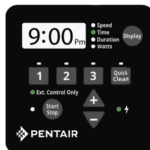
Figure 12: Activating External Control Only
