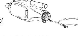
2. Connect the USB charging cable to the charging adaptor, then plug the charging adaptor to the power source.
